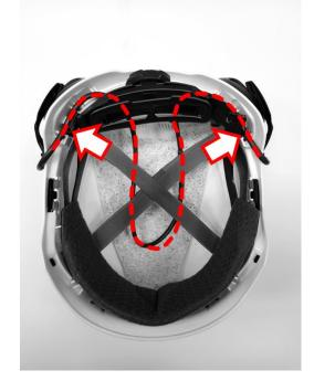
3. Make a loop of the cable and attach the cable at the mark to the head harness with the cable ties. Cut the cable tie.
